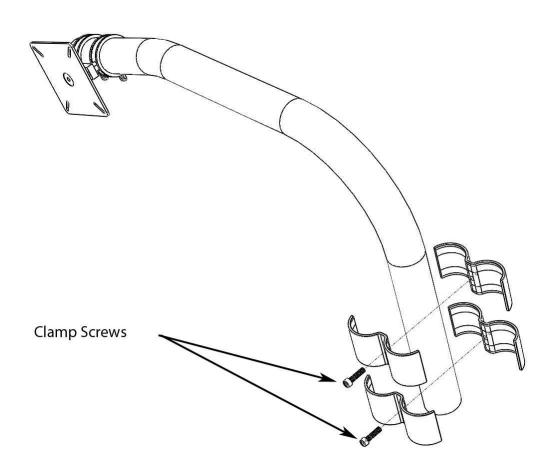
3) Ensure clamps are spaced a minimum of 3" apart and approximately 1" from the end of the tube to ensure a stable mounting position.
