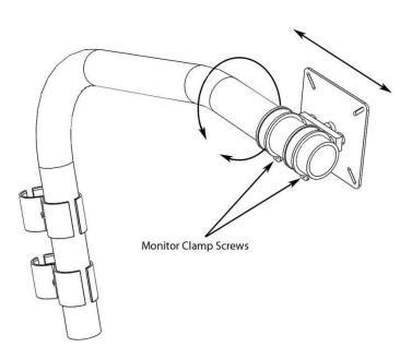
5) Loosening the lock nut shown below, will allow you to pivot the monitor mount plate a full 360 degrees to allow for the monitor alignment of your choosing.
