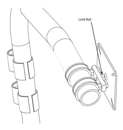
6) Please try to mirror the mounting position as closely as possible on the right hand side of the Dreamflyer machine. This will ensure that the symmetrical balance is maintained therefore requiring little or no compensation in the counterweight set up. (See next chapter).
