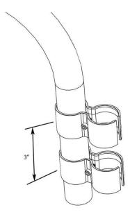
4) Loosening of the two monitor clamp screws will allow you to slide the monitor in and out along the tube as well as swivel it around the tube for the right angle.
